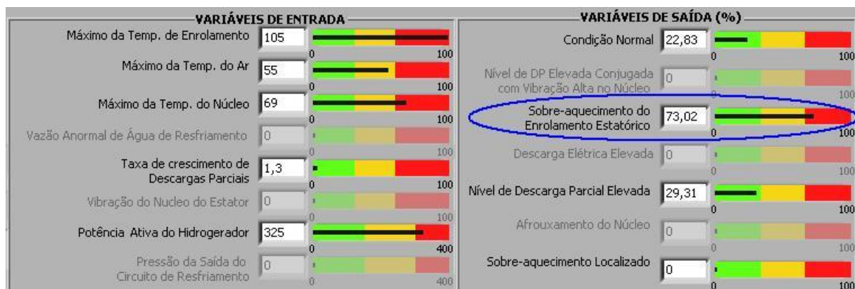
Figure 6 - Failure of overheating of the stator winding found
