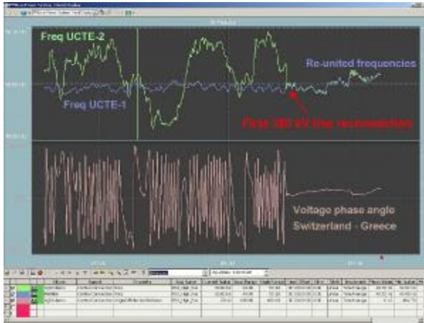
Fig.11: WAMS on-line trend display: UCTE-1 and -2 voltage phase angle difference and frequencies during the historical resynchronization process
