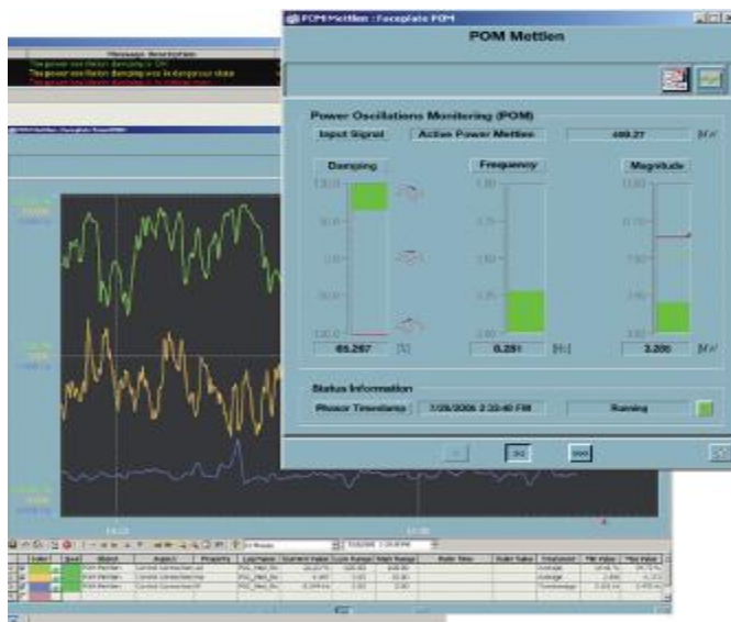
Figure 2: Power oscillation monitoring with the graphical user interface
