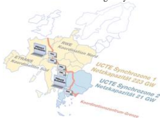
Fig. 8: WAMS, with installations in Switzerland, Croatia and Greece, is used for supervising of system stability and recording power system dynamics during and after the resynchronization.
