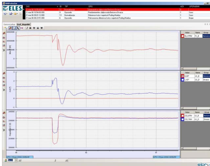
Figure 8: Real-time data display of active power, phase angle and voltage profile
